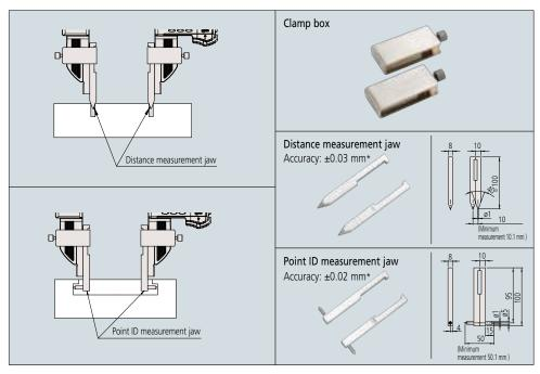
\* Accuracies shown in the diagrams are of each accessory and accuracy resulting in mounting them on the main body is not guaranteed.
